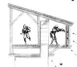
century, its floor had trap doors through which the defenders could protect the foot of the keep wall by dropping projectiles on the assailants below. Later, this was replaced by a line of more robust **machicolations** (in stone), around the top of the keep. The hoardings gallery was reconstructed as part of the restoration work on the château.
